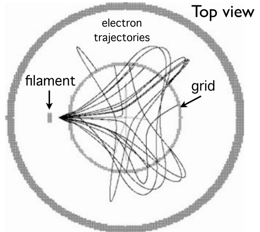
***- ionization and detection efficiency depends on electric fields inside sensor. Mechanical changes cause calibration drift...***
