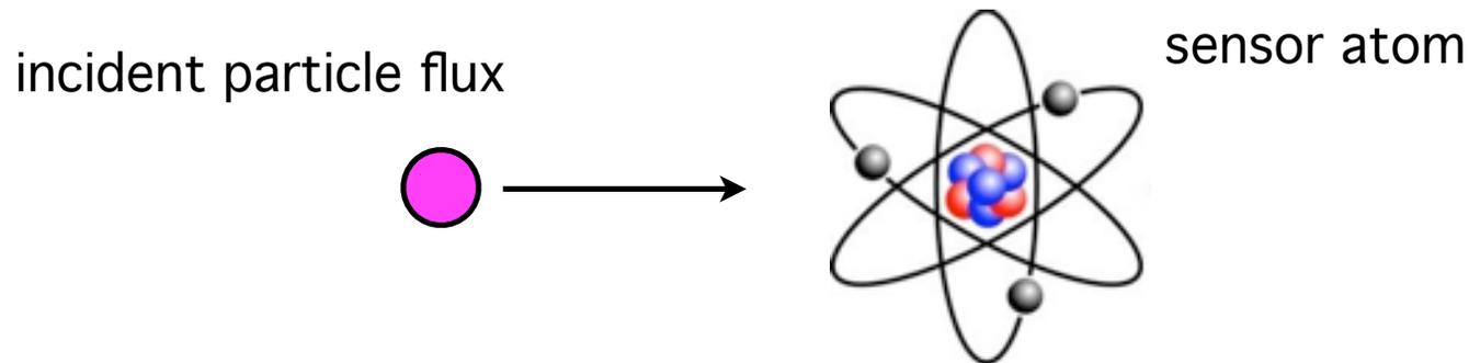
***a collision-induced state change of the sensor atom***
