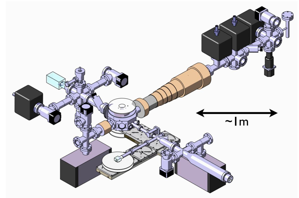
Typical flux for  ${}^6\text{Li}$  and  ${}^{40}\text{K}$ :  $\sim 10^9$  at/s
