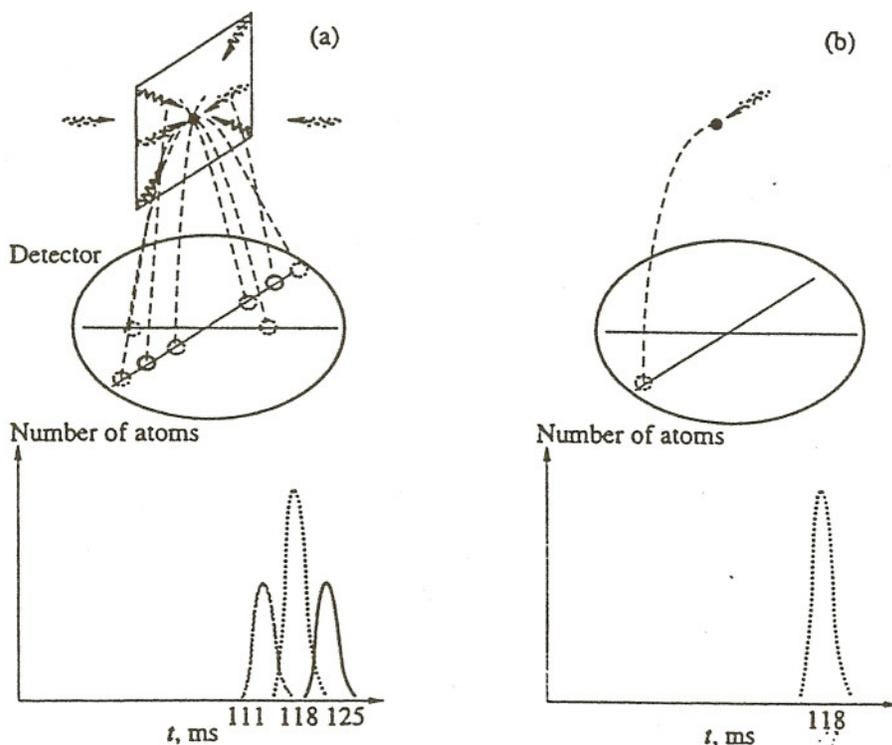
Fig. 3. Experimental scheme for 3D VSCPT cooling followed by adiabatic passage. (a) The system is initially prepared in a set of eight wavepackets which will follow ballistic trajectories to the detector. The time of flight distribution should show three peaks centered at 111, 118, and 125 ms. (b) Following adiabatic passage, the single wavepacket should manifest itself as a single detected spot and a single temporal peak.
