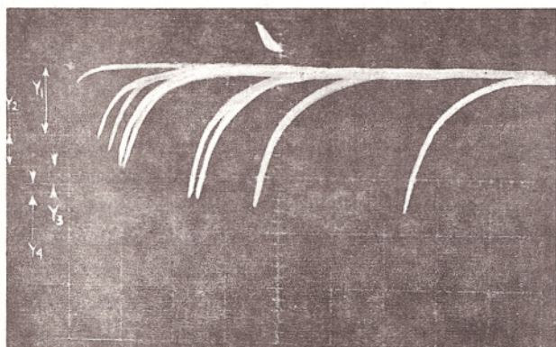
Fig. 16. Transient signals of light transmitted by Rb vapour. Construction of the T_1 -relaxation curve (FRANZEN [1959]).
