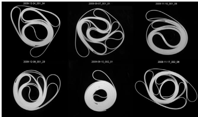
Fig. 2: Panel of folded configurations resulting from experiments with the same parameters. The rod is prepared in the initial configuration (fig. 1(a)) then the rotation frequency is increased from 0 to 12 Hz in approximately 3 s. The large variety of geometry shows that the folding is a non-deterministic process.
