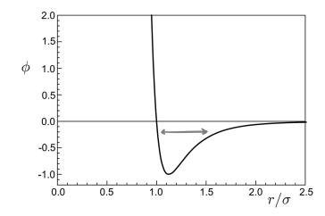
Fig. 4. Lennard-Jones intermolecular potential  $\phi$ . The interaction is strongly repulsive for intermolecular distances  $r < \sigma$ . At large distances, the molecules are attracted to one another. The gray arrow points to the presence of thermal fluctuations, which, in a liquid, lead to substantial variations of the intermolecular distance.
