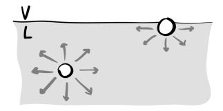
Fig. 1. Sketch showing the missing intermolecular bonds close to the liquidvapor interface, giving rise to an increase in the free energy per unit area, that is, the surface tension.
