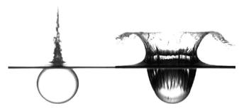
FIG. 42. The splash produced by a sphere impacting on water is caused by the contact line of the solid-air-water interface becoming unstable, so a sheet of water detaches from the solid. On the left, no instability occurs for a static contact angle of  $\theta_{\rm eq}$ =15°, while for  $\theta_{\rm eq}$ =100° (right) a splash is produced. From Duez *et al.*, 2007.
