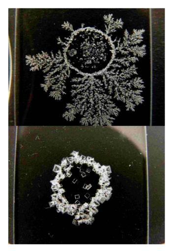
FIG. 44. (Color online) Deposit from an evaporating droplet of two different salt solutions, top, Na<sub>2</sub>SO<sub>4</sub>, bottom, NaCl. This shows that the wetting properties of the salt crystals are important for determining where crystals form. From Shahidzadeh *et al.*, 2008.
