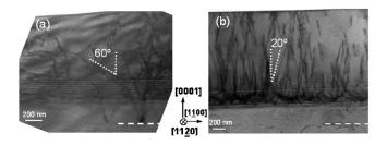
FIG. 3. Cross sectional TEM images of  $Al_{0.50}Ga_{0.50}N$  layers on single SL buffer. (a) Least relaxed sample (sample A). (b) Most relaxed sample (sample D). The dash lines indicate the beginning of AlN homoepitaxial layer.
