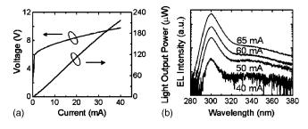
FIG. 4. Performance of deep UV LEDs on bulk AlN. (a) *L-I-V* characteristics of 50  $\mu$ m diameter device. (b) EL spectra with different currents (from 40 to 65 mA) for a 100  $\mu$ m diameter device.
