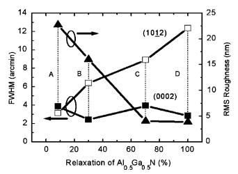
FIG. 2. Relations between surface RMS roughness (triangles) from AFM images ( $20 \times 20 \ \mu m^2$ ), FWHMs of XRD rocking curves along (0002) (solid squares), (1012) (open squares) diffractions, and the degree of strain relaxation for 1  $\mu$ m Al<sub>0.50</sub>Ga<sub>0.50</sub>N grown on single superlattice buffers.
