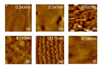
FIG. 1. (Color online) AFM images of high Al-content AlGaN superlattices on bulk AlN. The scan area of (a), (b), and (c) is  $10 \times 10 \ \mu m^2$  and (d), (e), and (f)  $1 \times 1 \ \mu m^2$ . (a) and (d), (b) and (e), and (e) and (f) are taken after the growth of superlattices 1, 2, and 3, respectively. Root-mean-square (rms) roughness from each scan is labeled.
