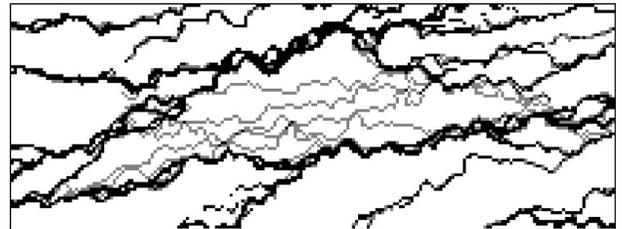
FIG. 6. Close-up look at an avalanche ( $\theta=10^\circ$ ,  $v=240 \mu\text{m/s}$ ). Successive positions of the CL are separated by 20 ms. The black curves are pinned configurations of the CL, defined as configurations where the CL stayed at least for two successive frames. The gray curves are instantaneous, unpinned configurations. (The actual size of the image is  $3.7 \times 1.4 \text{ mm}^2$ .)
