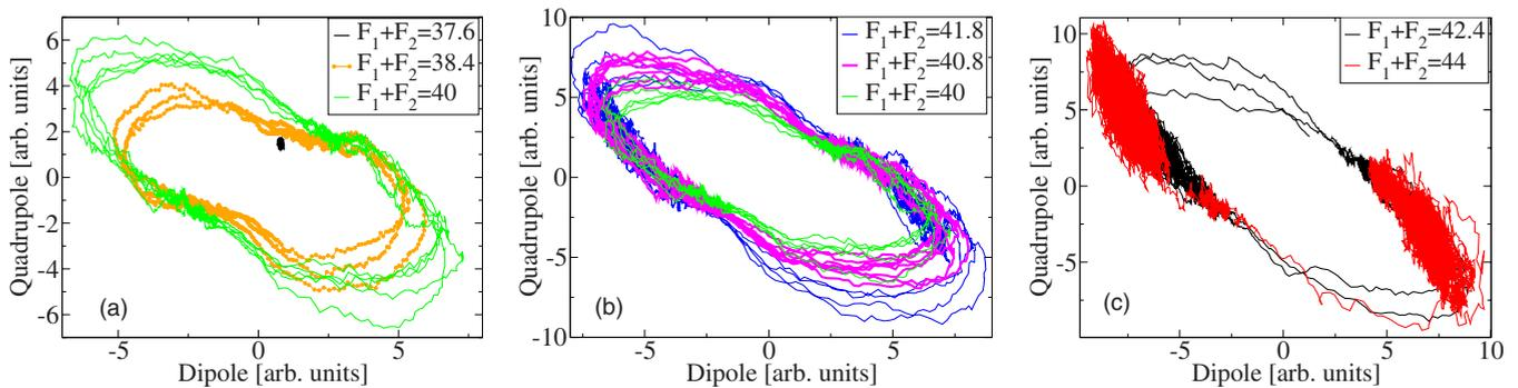
FIG. 4. (Color online) (a) Evolution of the magnetic field in the phase space  $(D, Q)$  at low frequencies: there exists a range of bistability in which a stationary dynamo (black dot) and a periodic limit cycle (orange circles) are both metastable. (b): Evolution of the limit cycle when  $F_1+F_2$  is increased from 40 to 41.8 Hz. (c) Chaotic reversals obtained for large values of  $F_1+F_2$  in the vicinity of a saddle-node bifurcation.
