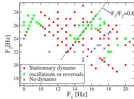
FIG. 2. (Color online) Parameter space: (cross) no dynamo, (circle) stationary dynamos, (star) oscillatory or random reversing dynamos.
