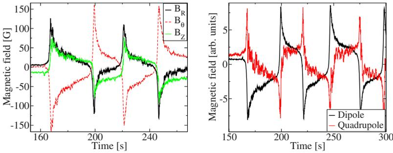
FIG. 3. (Color online) Top: time recordings of the three components of the magnetic field. The rotation frequencies are increased from 14.4/24 Hz to 15/25 Hz, leading to a transition from a stationary low amplitude dynamo regime to a limit cycle. Bottom: behavior of the dipolar and quadrupolar parts of the magnetic field. Note the transfer between the two components during reversals.
