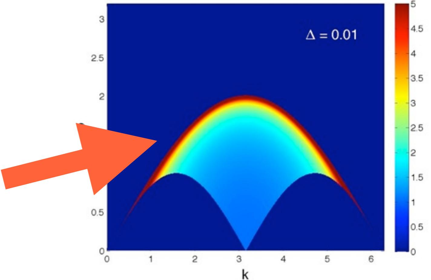
$$S_2^{zz}(k, \omega) \xrightarrow{\omega \rightarrow \omega_{2,u}(k)} f_u(\xi) \left( \sin \frac{k}{2} \right)^{-7/2} \sqrt{\omega_{2,u}(k) - \omega}$$
