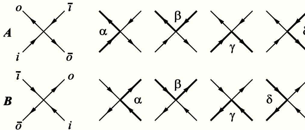
$$\begin{pmatrix} z_o \\ z_{\bar{o}} \end{pmatrix} = \mathcal{S} \begin{pmatrix} z_i \\ z_{\bar{i}} \end{pmatrix} = \begin{pmatrix} \alpha & \beta \\ \gamma & \delta \end{pmatrix} \begin{pmatrix} z_i \\ z_{\bar{i}} \end{pmatrix}$$
