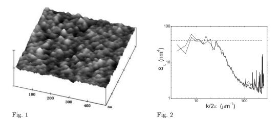
Fig. 1 – Atomic-force microscopy (AFM) picture of the etched Nb surface. The vertical scale is  $10\,\mathrm{nm}$  per division.
