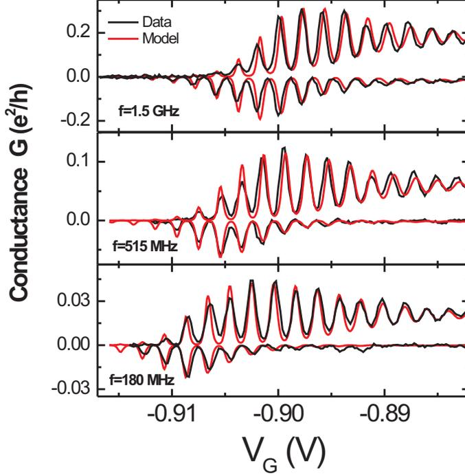
Figure 1: Complex conductance  $G$  of our sample as a function of the gate voltage  $V_G$  at  $T = 200$  mK for  $f = 0.18, 0.515$  and  $1.5$  GHz : Experimental results (black lines) and simulations (red lines). For clarity, we have plotted  $Im(G) > 0$  and  $-Re(G) < 0$ .
