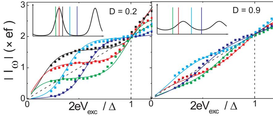
Figure 2:  $|I_\omega|$  as a function of  $2eV_{exc}/\Delta$  for different dot potentials at  $D \approx 0.2$  (left) and  $D \approx 0.9$  (right). Points correspond to experimental values and lines to theoretical predictions. Insets: schematic representation of the dot density of states  $N(\epsilon)$
