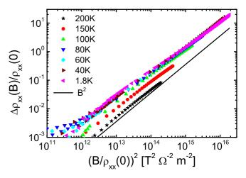
FIG. 6. Magnetoresistance  $\Delta \rho / \rho (B = 0)$  plotted as a function of  $B^2 / \rho^2 (B = 0)$ . Note the deviation from the Kohler's rule at high temperature.
