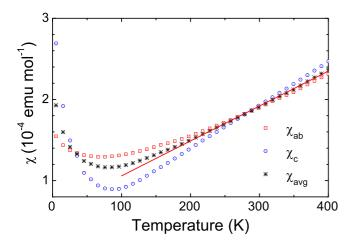
FIG. 3. Magnetic susceptibility of a BaNiS<sub>2</sub> single crystal.  $\chi_{ab}$  and  $\chi_c$  indicate the measurements taken with field in the *ab* plane and along the *c* axis, respectively. The average is given by  $\chi_{avg} = \frac{2}{3}\chi_{ab} + \frac{1}{3}\chi_c$ . The data have been corrected from the core diamagnetic susceptibility estimated to be  $\chi_{core} \approx -1.2 \times 10^{-4}$  emu mol<sup>-1</sup>.
