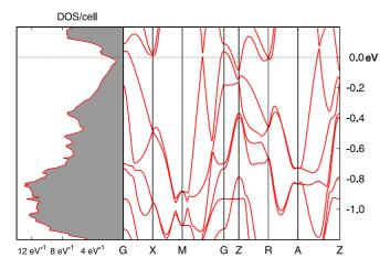
FIG. 9. Calculated electronic bands and total density of states. The dotted line indicates the Fermi level,  $\epsilon_F$ .
