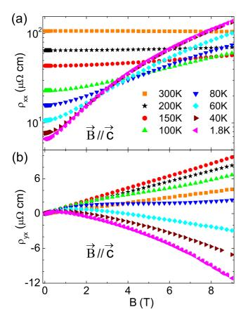
FIG. 5. (a) Transverse and (b) longitudinal magnetoresistivity of a BaNiS<sub>2</sub> single crystal with RRR = 15.8 at temperatures ranging from 1.8–300 K. The magnetic field was applied perpendicular to the current.
