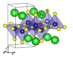
FIG. 1. Tetragonal structure of BaNiS<sub>2</sub>. The unit cell is drawn using solid lines.
