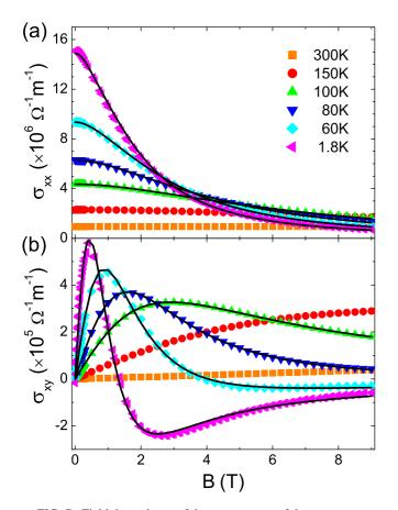
FIG. 7. Field dependence of the components of the magnetoconductivity tensor, (a)  $\sigma_{xx}$  and (b)  $\sigma_{xy}$ . Black solid lines are fits of the curves using Eqs. (3), (4) and a three-band model with two hole bands and one electron band.
