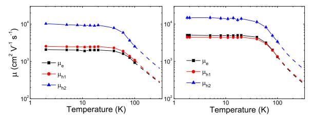
FIG. 8. Carrier mobilities extracted from the analysis of the temperature and field dependence of the longitudinal and transverse conductivity for two BaNiS<sub>2</sub> samples with RRR = 7.9 (left) and RRR = 15.8 (right). The dashed lines above 100 K indicate the extrapolated behavior of the mobility by assuming a conventional  $\mu_i \propto 1/T$  dependence expected for a metal with  $\rho \propto T$ .
