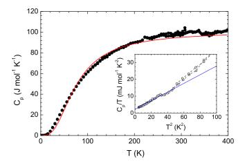
FIG. 2. Temperature dependence of the isobaric specific heat,  $C_P$ , of a bunch of BaNiS<sub>2</sub> single crystals. In the inset, the broken line is a fit of the low-temperature data that yields  $\gamma$  and  $\Theta_D$ . The red solid line is the theoretical Debye curve described by Eq. (1).
