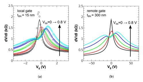
**Figure 5.** (a) Small signal resistance of the transistor obtained from the model (solid lines) and from the measured scattering parameters of sample-A at 2 GHz (circles). (b) Small signal resistance simulated for a remote gate transistor (h-BN dielectric thickness of 300 nm). The saturation effect is enhanced for the local gate device in the n-doping regime.
