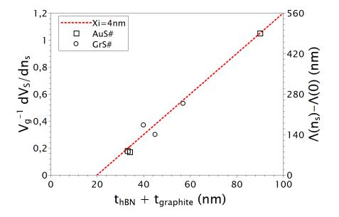
FIG. SI-8: Slope extracted from the linear increase of the ratio  $\frac{V_S}{V_g}$  as function of doping  $n_s$  (left axis), plotted with respect to the sum of hBN and graphite thicknesses for the 6 devices. Right axis gives the associated value of the junction length  $\Lambda(n_s)$ . The red dotted line is a linear fit corresponding to  $\xi = 4nm$ .
