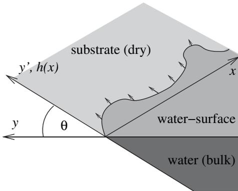
FIG. 1. The geometry of the contact line.
