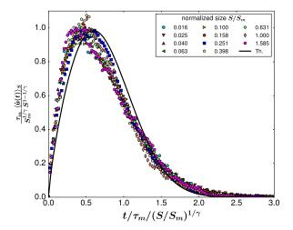
FIG. 6. Scaling collapse of the average shape at fixed avalanche sizes  $\langle \dot{\mathbf{u}}(t) \rangle_S$  in the FeCoB ribbon using the theoretical values of  $\gamma$  and  $\tau_m$ , as in Fig. 2. The collapse deviates from the universal functions predicted for SR systems (continuous black line) in the absence of eddy currents.
