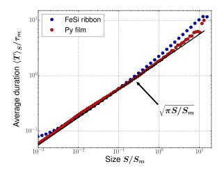
FIG. 3. Normalized average duration  $\langle T \rangle_S / \tau_m$  of avalanches in the FeSi ribbon (blue dots) and the Py thin film (red dots) as a function of the normalized size  $S/S_m$ . The continuous line is the theoretical prediction of Eq. (6).
