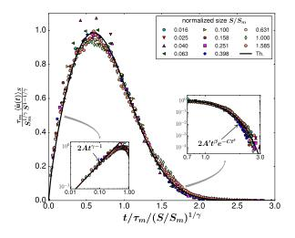
FIG. 5. Scaling collapse of the average shape at fixed avalanche sizes  $\langle \dot{u}(t) \rangle_S$ , according to Eq. (7), in the FeSiB thin film. The continuous line is the prediction for the universal SR scaling function of Eq. (9). The insets show comparisons of the tails of the data with the predicted asymptotic behaviors of Eqs. (10) and (11), setting  $\epsilon = 2$ , with A = 1.094, A' = 1.1,  $\beta = 0.89$ , C = 1.15, and  $\delta = 2.22$ .
