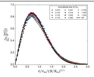
FIG. 4. Scaling collapse of the average shapes at fixed avalanche sizes  $\langle \dot{u}(t) \rangle_S$ , according to Eq. (7), in the Py thin film. The continuous line is the mean-field universal scaling function in Eq. (8).
