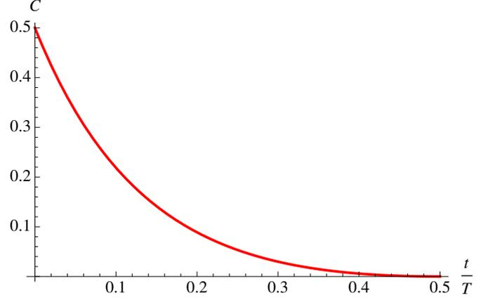
FIG. 5: The velocity correlation  $C(t, T)$  of Eq. (164) for  $T = 1$ .
